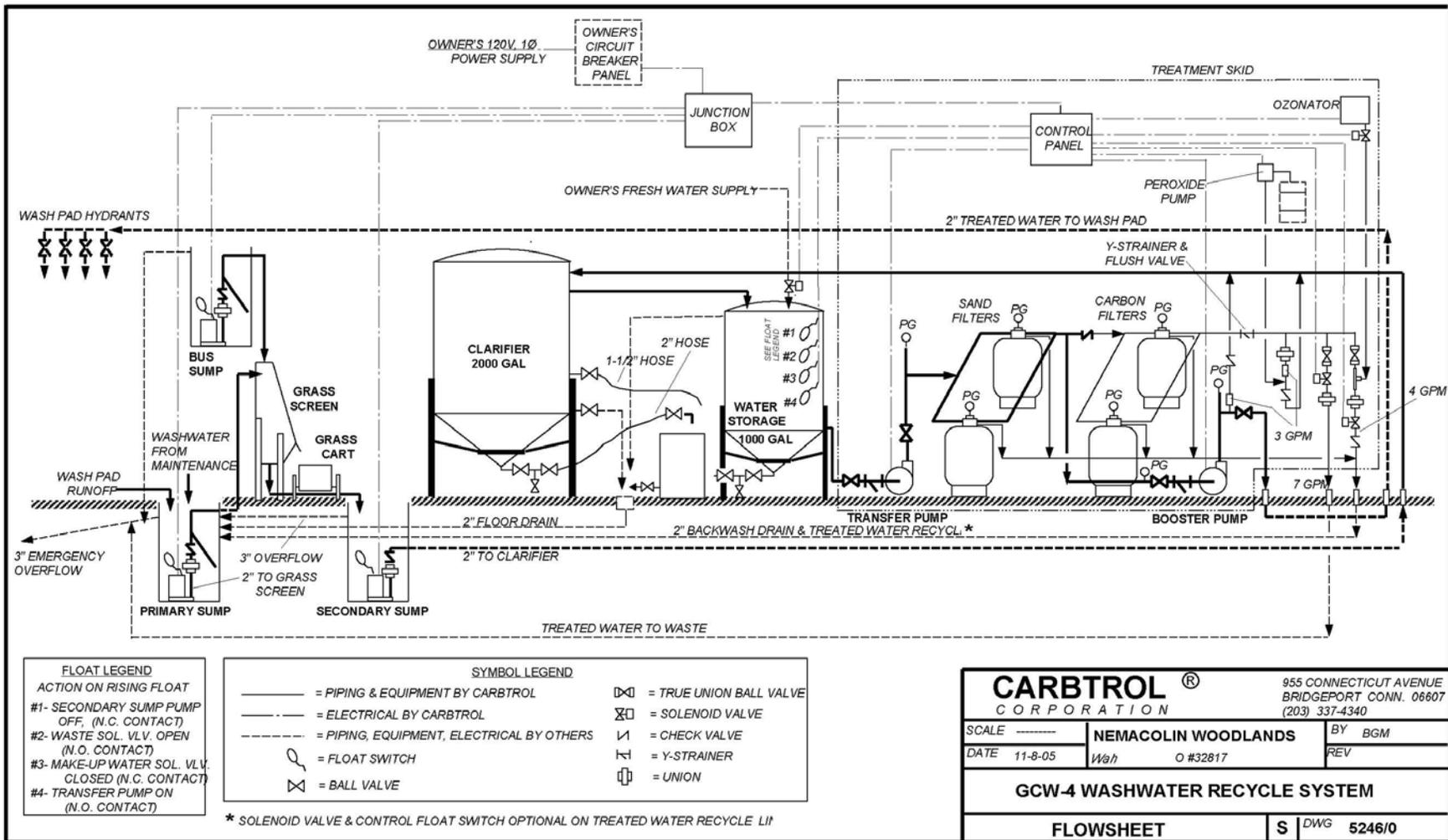
Figure I – Wash Water Recycle System
